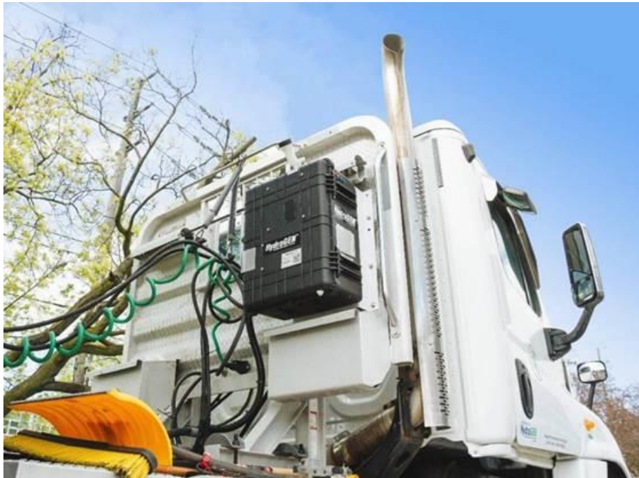
Figure 4: An after-market HydraGen unit installed on a Class 8 truck
