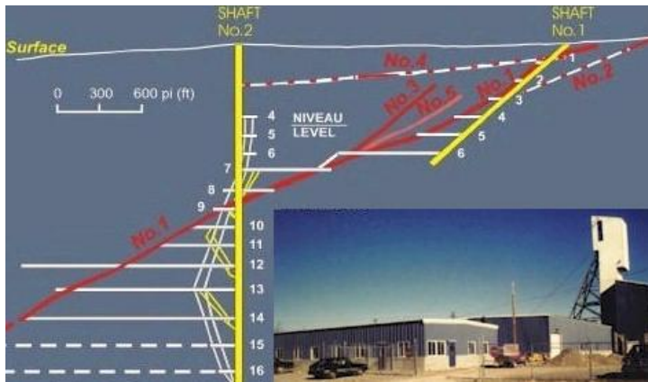
Figure 1. Elder Gold Project: 2,600-ft shaft, 16 levels, with functional surface buildings and underground equipment near-ready to go.
